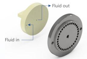
The flow path in the valve rotor is specifically designed with a hidden channel so that the sample liquid has minimum contact with the stator surface when the valve is turning. This feature is very effective in avoiding contamination of sticky compounds (such as benzopyrene) on the stator surface.
