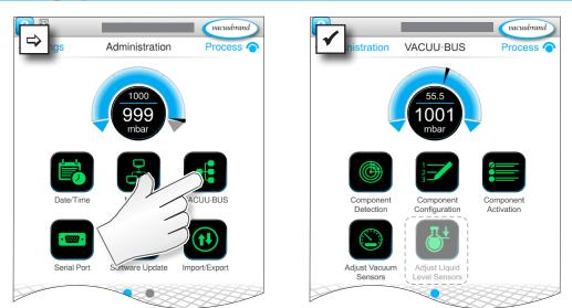
The buttons retrieve context menus. The context menus facilitate the use of presettings for VACUU·BUS components, e.g., address configuration, detection of connected components. Vacuum sensors and level sensors, amongst others, can be calibrated in this submenu.
