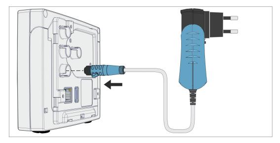
Power supply via plug-in power supply
