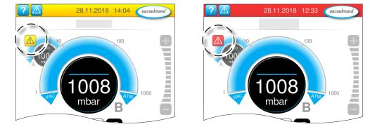
Warnings and / or errors are indicated by a flashing pressure curve. If the flashing pressure curve is pressed, the process with fault can be called up. The process without fault continues operation. If both processes are affected by the fault, both processes stop.
