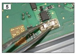
**5.** Insert the new fuse into the base.
