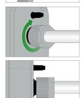
**Required connection material:** Union nut M14x1, sealing ring, PTFE hose.
