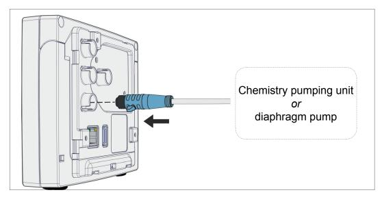
Controller power supply via peripheral device
