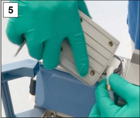
5. If all valves are correctly positioned, first insert the molded hose.
