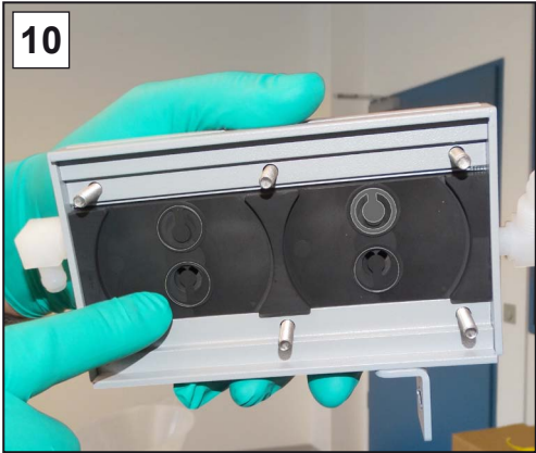
8. Check the housing cover for sticking valves and place the housing cover with the screw connections on the side.
