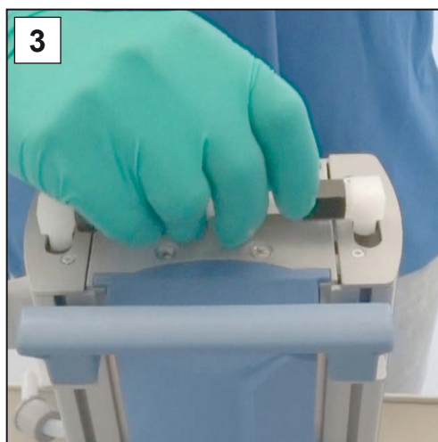
3. Tighten the knurled nut hand-tight; fork wrench SW17.
