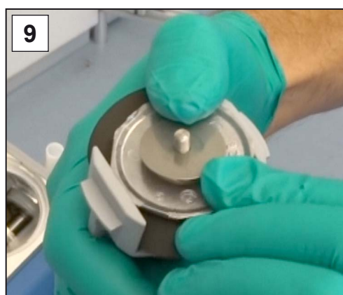
9. Fixate the diaphragm assembly in the diaphragm key.
