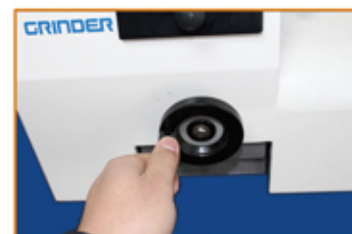
Turn the handle to set the gap
