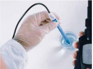
Special samples need special electrodes. SenTix® special electrodes can take on the challenges associated with measuring the pH value of surfaces, solids, suspensions, emulsions, low ionic samples, smallest volumes
