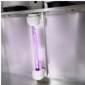
Air UV recirculation system in the chamber
